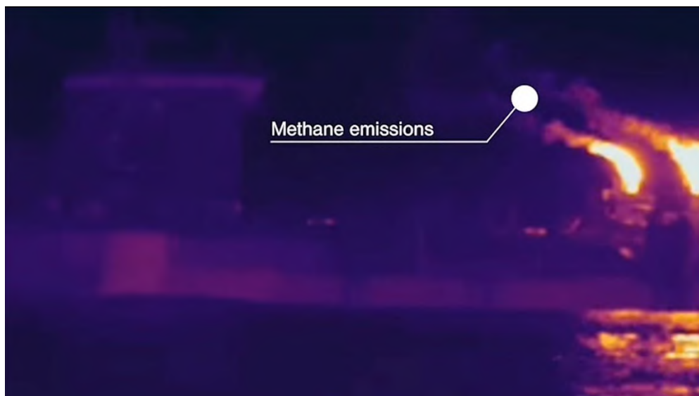
Infrared capture of methane emission from a cruise ship Source: The Cruise Ship Industry: A Floating Grave?
