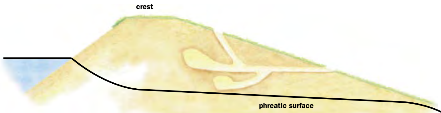
Figure 4-9. Groundhog burrows are extensive and irregular in pattern.
