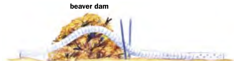
Figure 5-12. Massachusetts Beaver Pond Leveler
