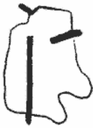
Fiber protrusion <5:1 Aspect Ratio
