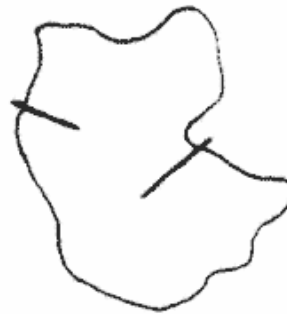
Fiber protrusion <0.5 micrometer
