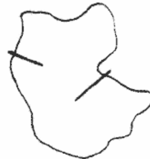
Fiber protrusion <0.5 micrometer
