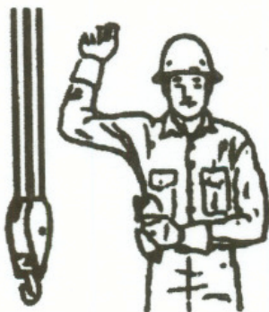
TRAVEL. (One Side Track). Lock the track on side indicated by raised fist. Travel opposite track indicated by circular motion of other fist, rotated vertically in front of body (for land cranes only).
