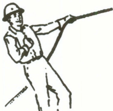
EXTEND BOOM (Telescoping Boom). One-hand signal. Hold one fist in front of chest, thumb tapping chest.
