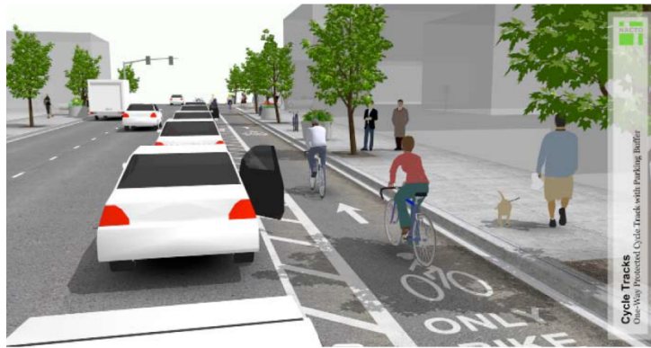
Figure B-E-9: Illustration of a Separated Bike Lane. A bike lane located between on-street parking and the curb is a Separated Bike Lane. Image Source: NACTO Urban Bikeway Design Guide.
