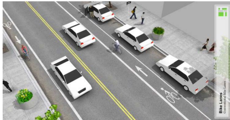
Figure B-E-10: Illustration of Conventional Bike Lanes. They can be located adjacent to the curb if there is no on-street parking, or adjacent to on-street parking. Image Source: NACTO Urban Bikeway Design Guide.
