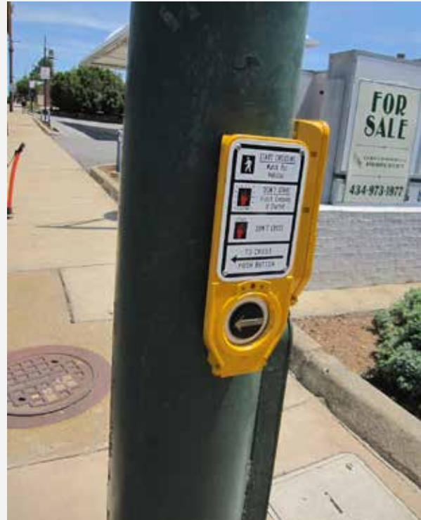
Figure 82: Activated APS Push-Button. This traffic signal is activated, meaning pedestrians push the black button to call a pedestrian phase to cross the street. It is also an APS that speaks the name of the street and vibrates when the pedestrian phase is on.
