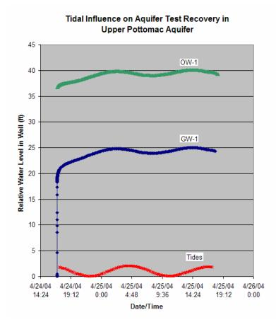
Note: This is an illustration of tidal effects during an aquifer test. This graph shows that tides at the tidal reference station do not necessarily correspond directly in time with the tides seen at the well. It is imperative that tides are observed in wells for multiple days, so as to be able to predict the onset of high or low tide in wells.
