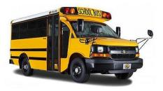
**Type "A"** school bus is a conversion bus constructed utilizing a cutaway front-section vehicle with a left side driver's door. This definition includes two classifications: Type A1, with Gross Vehicle Weight Rating (GVWR) 14,500 pounds or less; and Type A2 with a GVWR greater than 14,500 pounds but less than or equal to 21,500 pounds. Both Type A1 and A2 buses shall be equipped with dual rear wheels (DRW).
