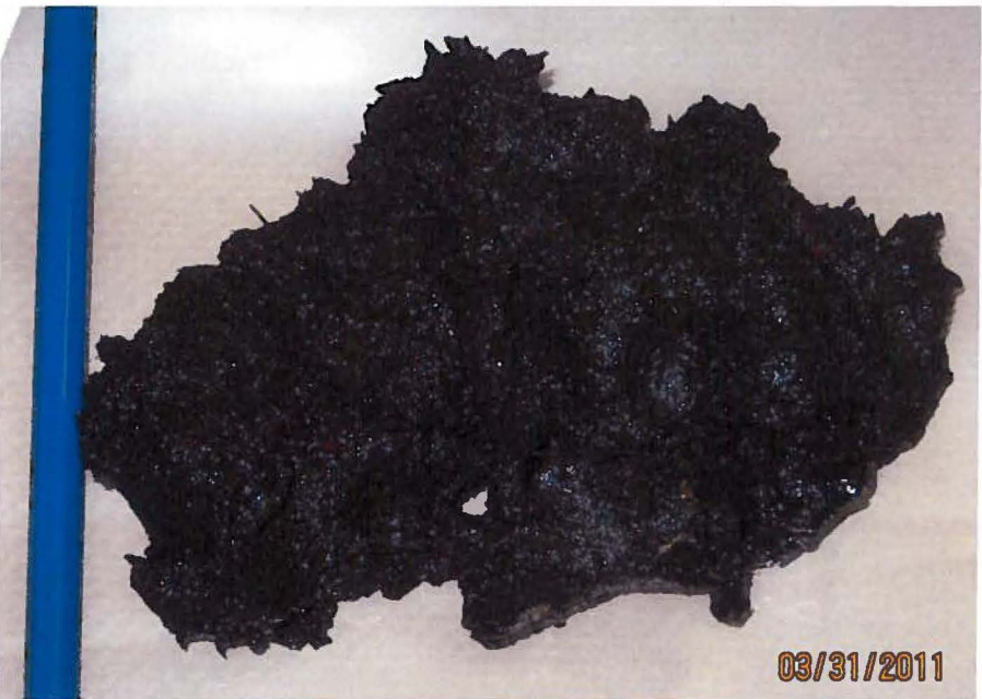
Photo 8. Degraded peat material sample in March, 2011, from Ecoflo unit in Saluda, VA.
