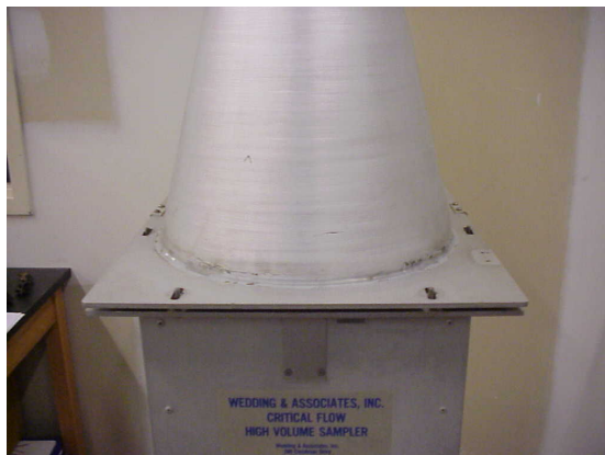
Inlet set on sampler base
