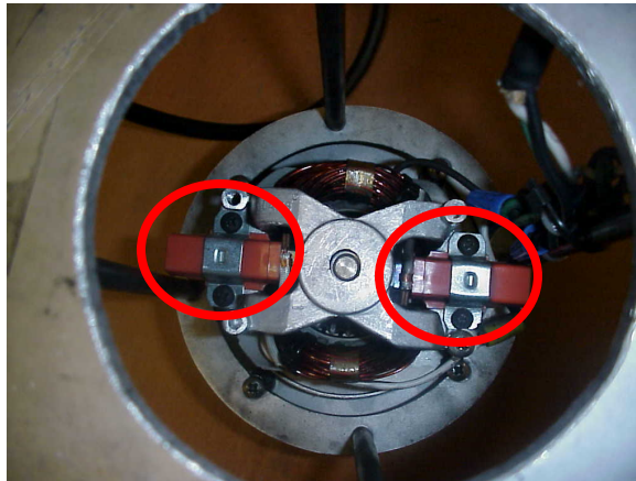
Note retaining clips highlighted above.
