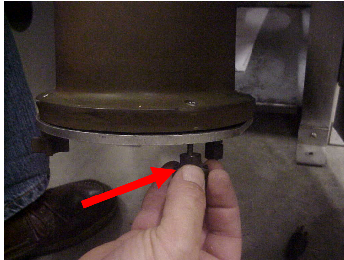
Motor Mount Flange plate wing nuts being installed
