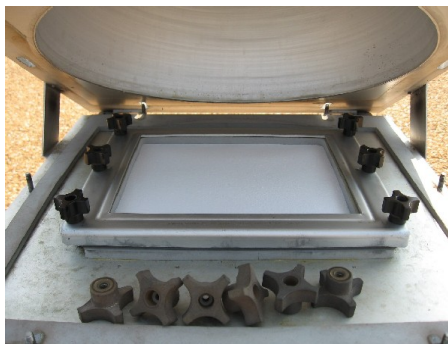
Exposed filter, wing nuts tight
