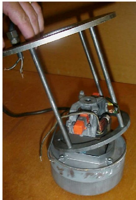
Note cage fits over motor
