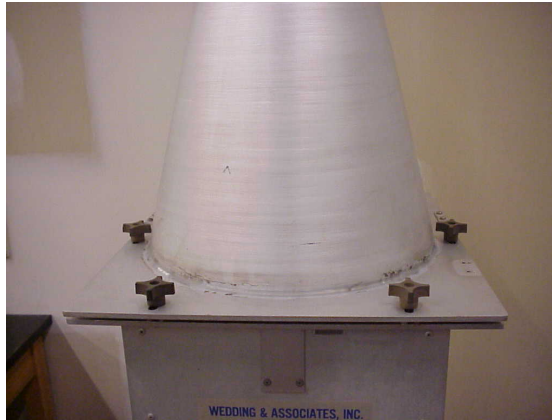
Inlet secured to sampler base
