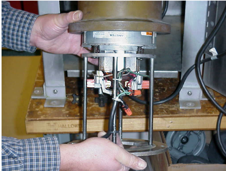
Motor assembly removal
