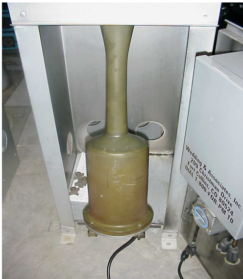
Critical Flow Device clear of assembly (front view)
