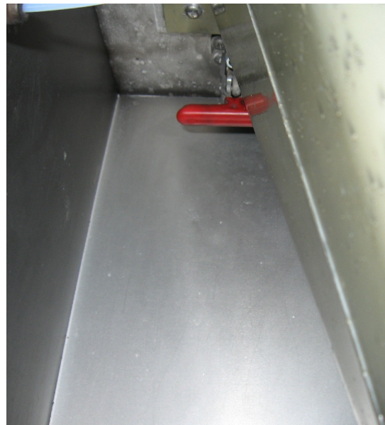
View of hold-down clamp when CFD is in normal operating condition
