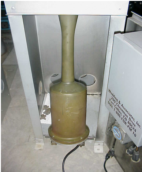
Critical Flow Device clear of assembly (front view)
