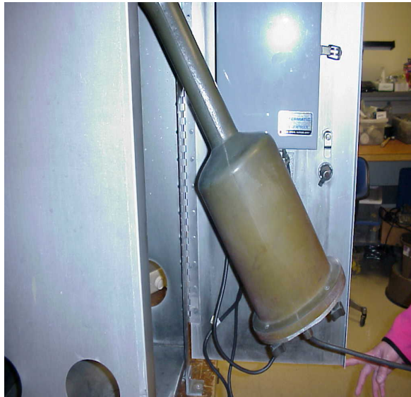
Critical Flow Device clear of assembly (side view)
