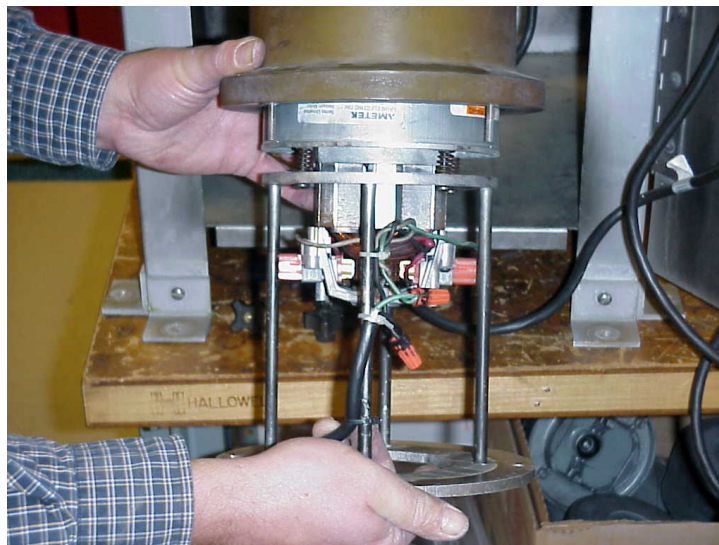
Motor assembly being put into the CFD
