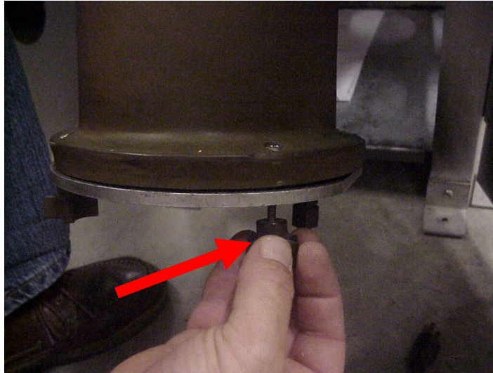
Motor Mount Flange plate wing nuts
