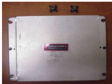
Cassette with wing nuts removed
