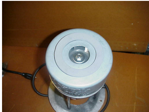
Completed gasket installation
