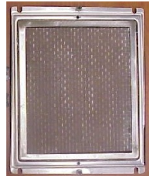
Lower cassette plate with filter support screen
